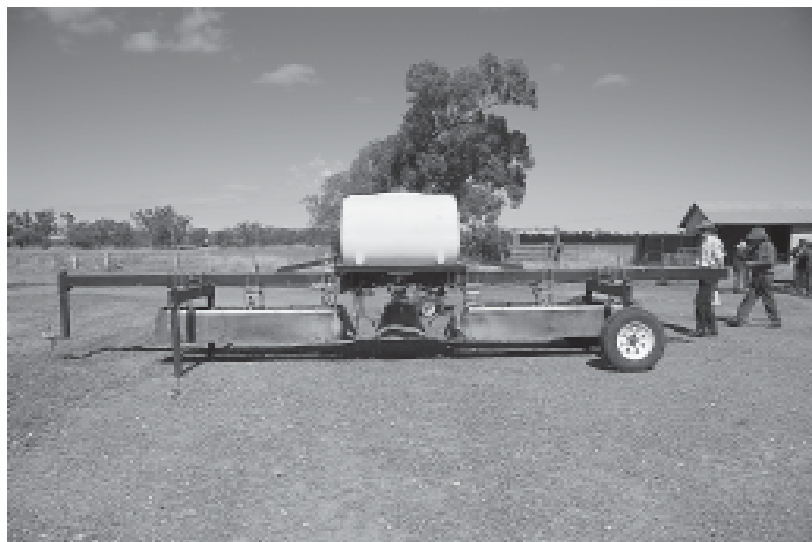
Shielded rig for spraying herbicide around twin rows of leucaena.
