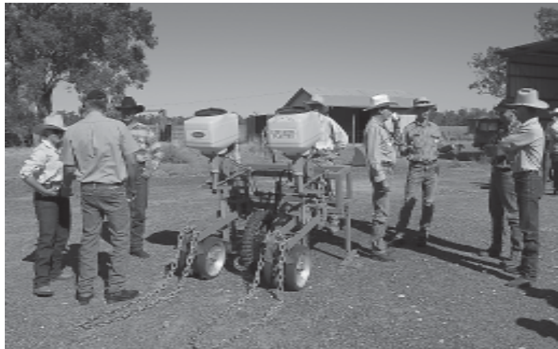
Twin row precision planter with side press wheels and covering chains.
