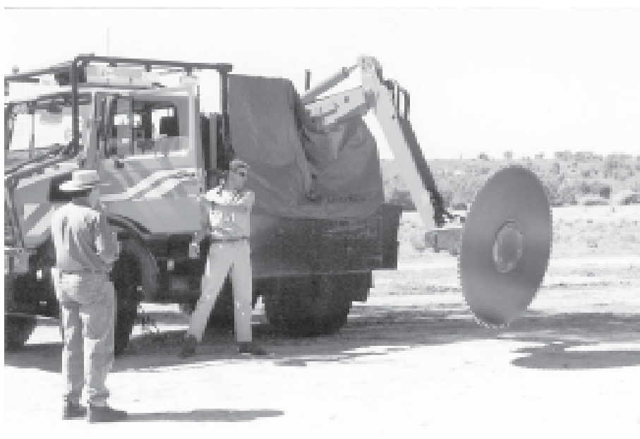
5-ft circular saw to cut back tall tagasaste. (Call that little Critter a knife, Peter?)
