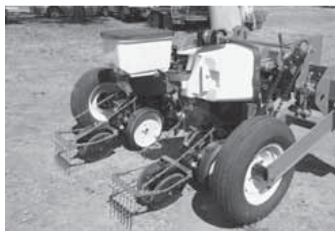
(Above) The Norseman Techni-Plant is a precision seeder for leucaena.
