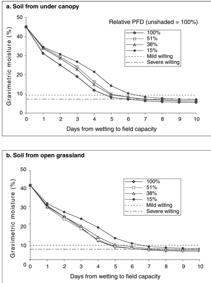
**Figure 2.** Drying curves for soil for the 4th 10-day drying cycle under 4 different shade treatments for: a) soil collected from under the canopy of *S. saman*; and b) soil collected from the open grassland. The gravimetric soil moisture ( $\theta_g$ ) at which mild and severe wilting occurred is indicated by the dotted lines.
